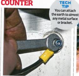
The tachometer has four wires: +12V; earth; wire to coll; a wire to the instrument lighting. Use crimp terminals or Scotchlok-type connectors. Start by attaching the earth wire to the bulkhead.
