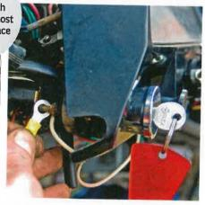
Attach the positive wire Join the positive wire to any accessory circuit that's only live when the ignition's on – or join it directly to the output terminal of the ignition switch. It's a good idea to fit an in-line fuse (3A or 5A).
