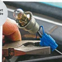
The backlight of the rev counter needs to be spliced into the instrument lighting. Some backlights have two wires – supply and earth. Others have one wire and share the earth with the rev counter.
