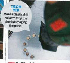
If you're drilling holes in the dash, centrepunch them first. To make a large hole to house the counter, chain-drill 6mm holes around the outline then cut and file it smooth. Or use a hole saw.
